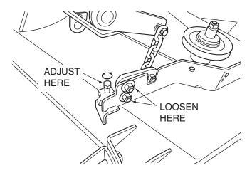
Figure 6-5. Cutter Deck Level Adjustment
